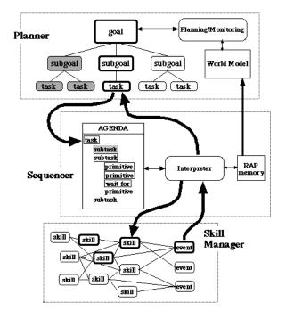
Figure 1: The 3T intelligent reactive control architecture.
