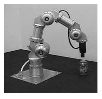
Figure 2: The six DOF manipulator designed for the project.
