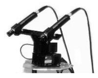
Figure 3: The vision system cameras and head.
