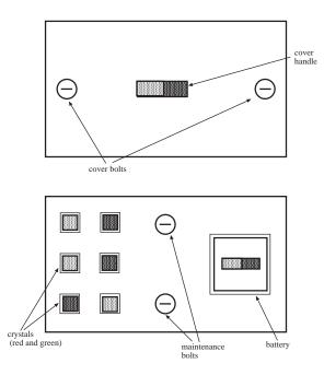
Figure 1: The experiment bay, or TaskBoard, used in our scenario. The top part of the figure shows the hard cover that sits on top of the bay. The bottom part of the figure shows the experimental area.
