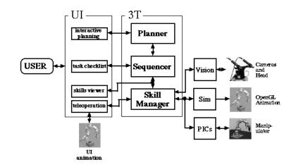
Figure 4: Overview of the software modules for traded control and for our specific TaskBoard scenario.
