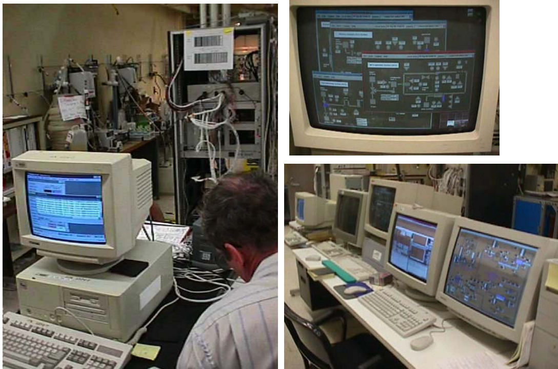
Figure 7 3T Control Computers for the iWRS. On the left is a view of the 3T VME Rack behind the computer that is used as a secondary interface to the RO high-pressure pump. On the right is a view of the (unattended) 3T control table. From foreground to back, the displays are two sequencer/planner displays, the IPC/skill manager display, the display of the broadcast server, and a display associated with the high-pressure pump used in the RO. In the upper right is the display showing the graphical user interfaces (GUIs) for each subsystem generated by the data broadcast from each skill manager.
