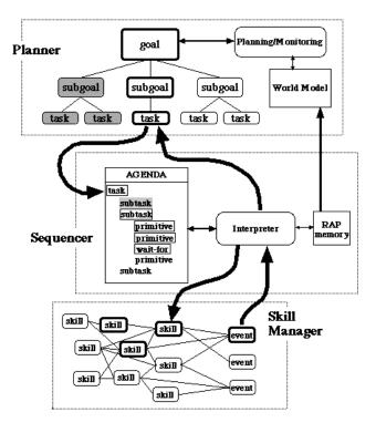
Figure 1: A layered architecture for intelligent control.
