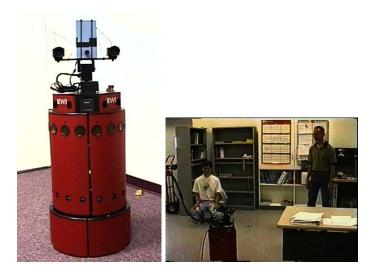
Fig. 6. Left: Our mobile robot with a stereo pair of camera and a single color camera. Right: The robot attending to two different people.
