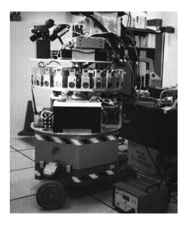
Figure 4: The stereo vision system is mounted on top of our robot; the sonar sensors are just below it.
