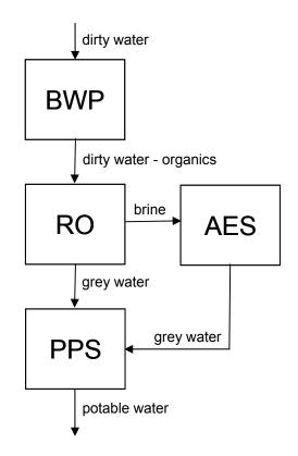
Figure 3: The Water Recovery System
