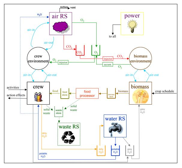
Figure 1: The various modules that comprise the integrated simulation
