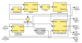
Figure 4: Matlab/Simulink model for the BWP.
