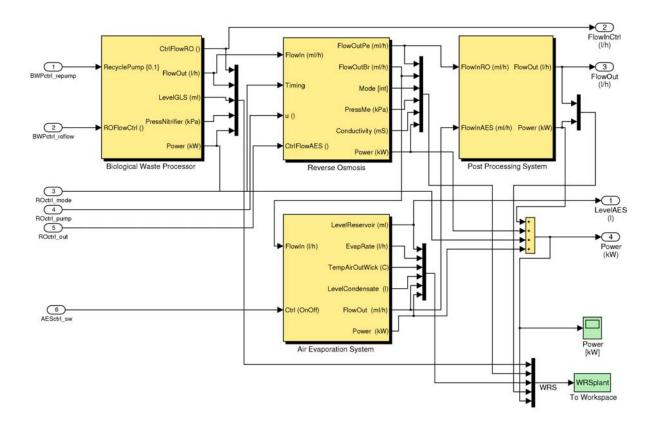
Figure 7: Matlab/Simulink model of the WRS. Many more measurements are available on the system dynamics than are exposed to the model interface.
