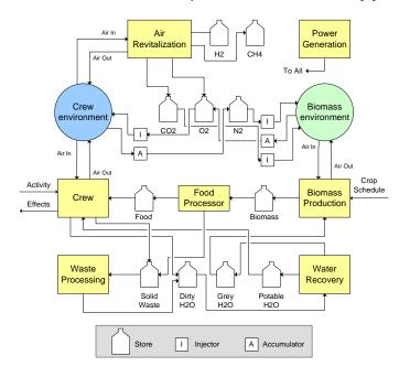
Figure 1: Diagram of a generic advanced life support system implemented as a BioSim model.
