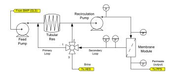
Figure 5: Diagram of the RO system.
