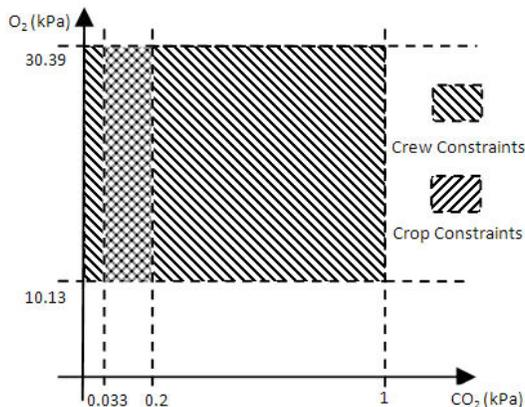
Figure 2. Atmospheric constraints on workable system states
