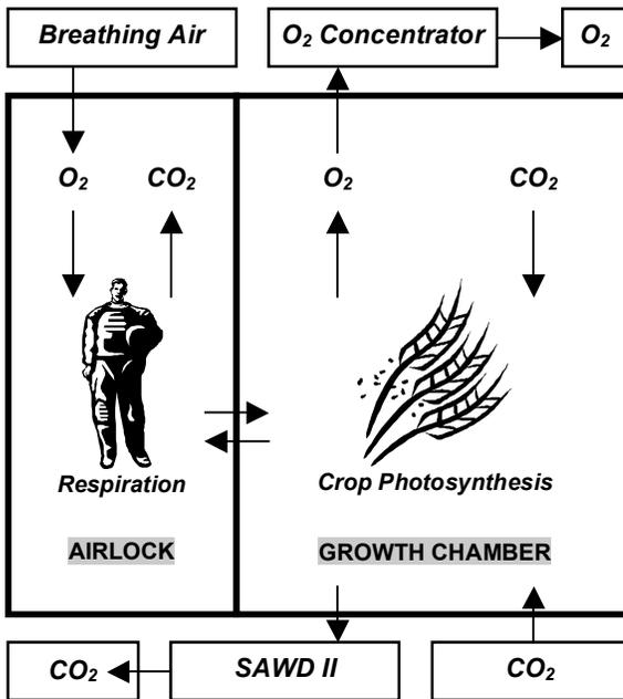
Figure 1. Schematic representation of oxygen and carbon dioxide exchange during the test.
