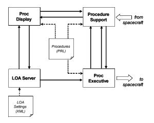
Figure 1. Adjustable Autonomy Architecture
