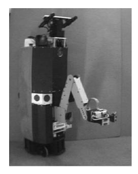
Figure 4: Chip with color vision system and manipulator
